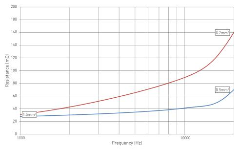
Figure 6. Graph of resistance versus frequency for QED power cables Standard cable (—), QED XT5 power cable (—)
